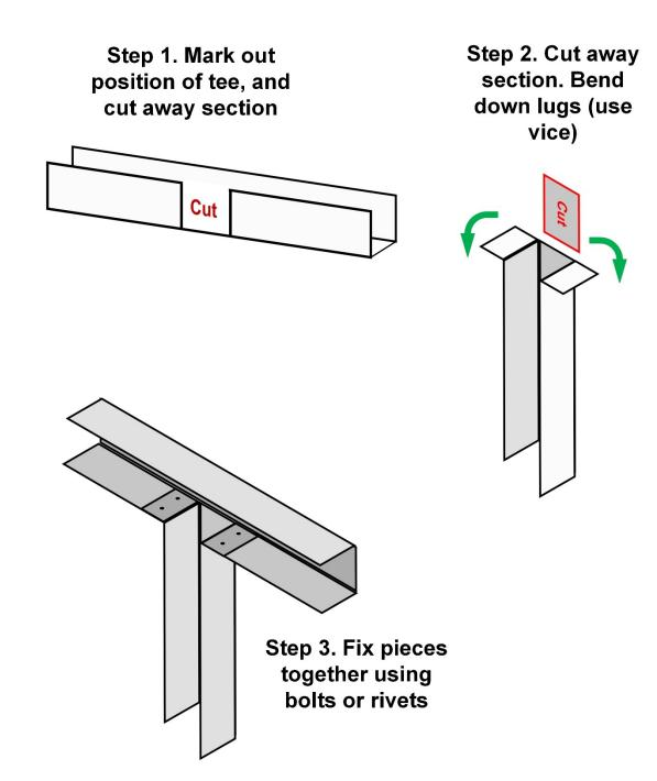
Notes: Ensure to file cut edges smooth after cutting. Use blocks of wood to support trunking in vice during cutting in step 1.
